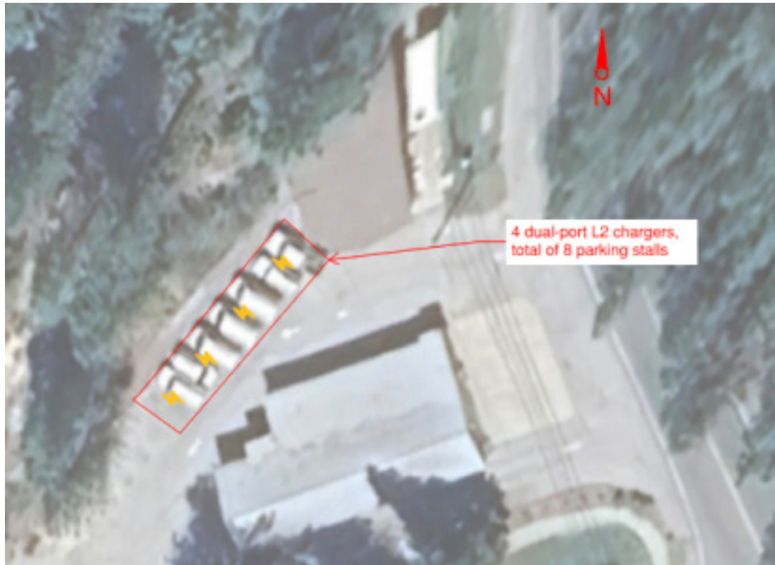
Figure 19: Recommended Charger Locations for Facilities SC
