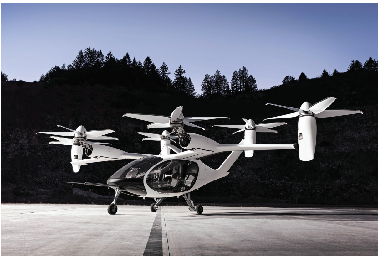
FIGURE 2.1 Self-flying air taxi from Joby Aviation. It represents an example of a potential future air taxi vehicle. SOURCE: Joby Aviation's Aircraft in Santa Cruz, Calif., Joby Aviation, 2019.
