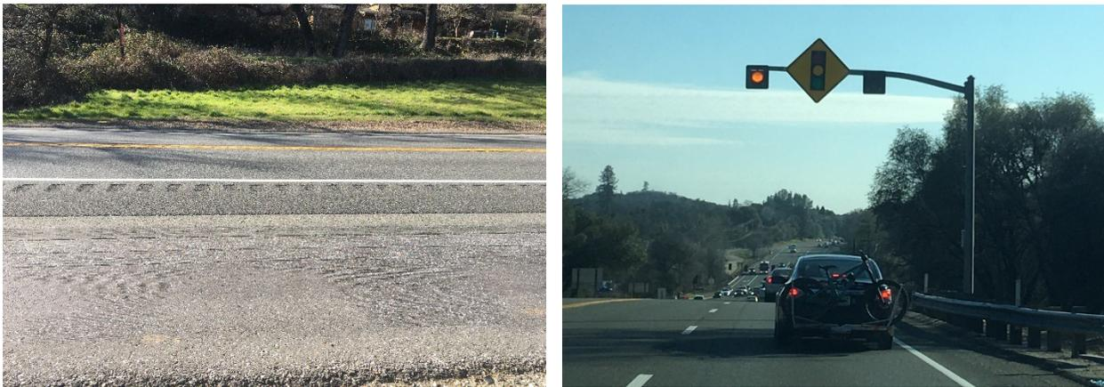
**Figure 9 – Edge Line Rumble Strip and Overhead Flashing Beacon**
