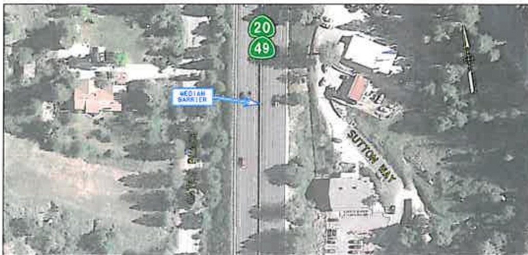
EXAMPLE OF AN EXISTING 22' MEDIAN WITH BARRIER APPROXIMATELY 4 MILES NORTH OF PROJECT IN GRASS VALLEY ON HIGHWAY 20/49 WITH FRONTAGE ROADS
