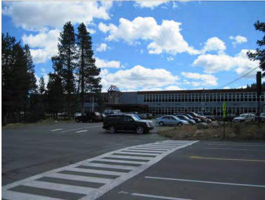
The pattern of paint in crosswalks can vary; yellow crosswalks denote a crosswalk near a school. The above striping pattern illustrates a "ladder" crosswalk.
